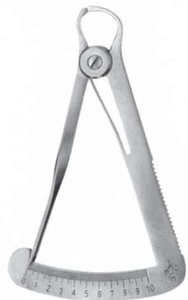
SS-2614 Fig. 2 Iwanson spring caliper For wax.
