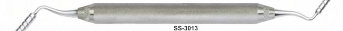
SS-3013 Titanium graft packer/ placement site depth gauge 3.3mm & 4.0mm Diameter tips Marked at 8, 11, 13, 15 & 18mm
